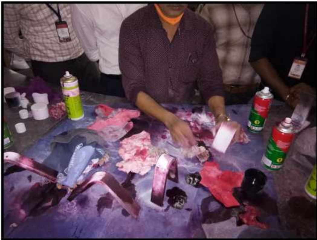
Dye Fluorescent penetration test demonstration
