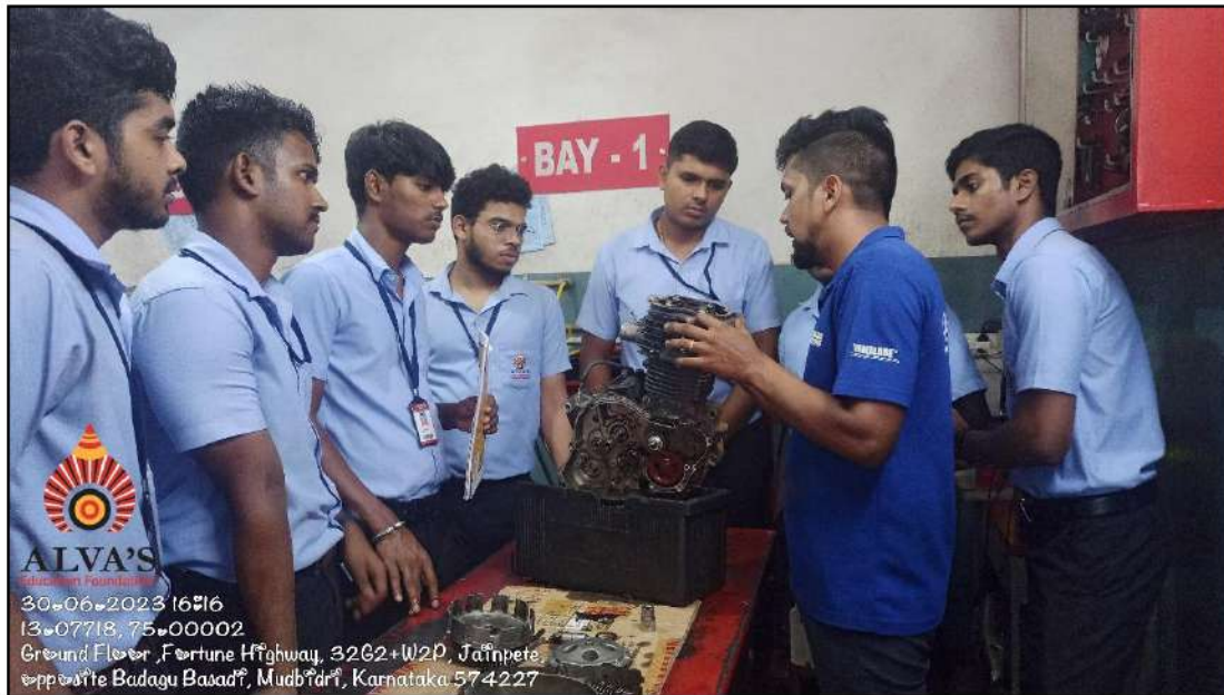
Assemble & disassemble of Yamaha Bike Engine.
