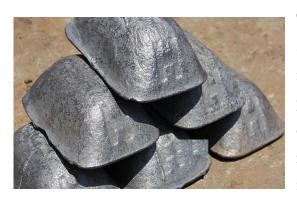
The demand for the international has a sharp rise, the total proton or pig iron. Pig Iron is an intermediary product of smelting iron ore with coke. It has a high carbon content ranging from 3.5 to 4.5%. Which makes it very brittle and not useful
