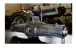
Kirloskar ferrous produce a variety of housings used in manufacturing tractors, commercial vehicles, industrial engines and construction equipment. The weight of these **castings ranges**
