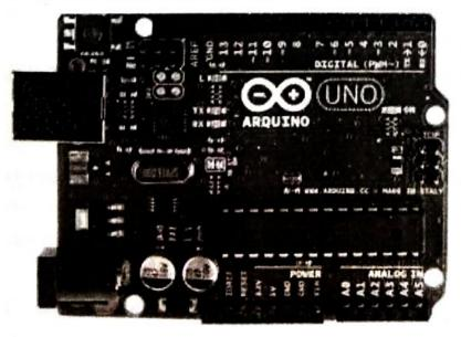
The Arduino board plays a central role in an IoT air and sound pollution monitoring system. It serves as the main microcontroller that interacts with sensors, processes data, establishes internet
