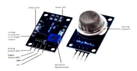
Fig 2.1:MQ-8 Hydrogen Gas Senso
